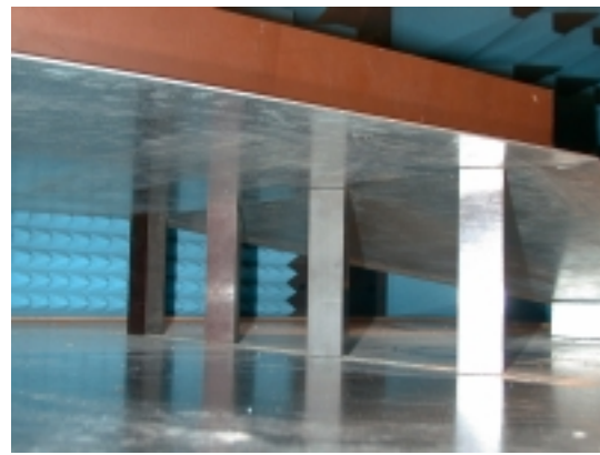
Figure 4: Stripline Modified Supports
